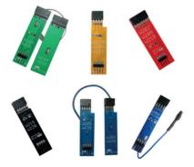
With help of Mercedes-Benz Test Kit, you do not need to test new programmed keys on the vehicle. Our user friendly PCBs will assist you to check new programmed keys on the bench.
