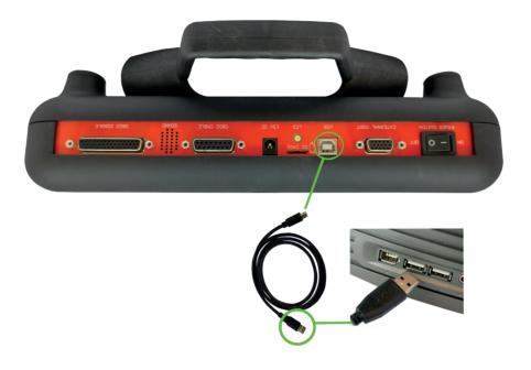
After establishing USB connection, select language and press "CONNECT" button to connect to PC software.
