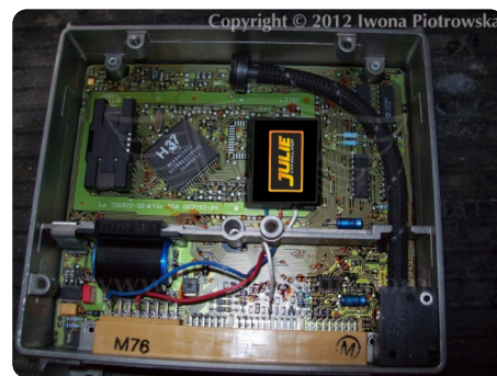
Although the picture shows Julie Emulator, the same way of connecting to ECU also applies to Clixe
