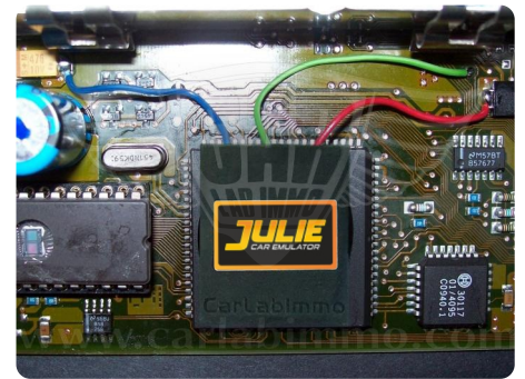
Although the picture shows Julie Emulator, the same way of connecting to ECU also applies to Clixe
