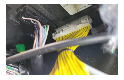
Below you may find picture with connections in Clio V, where the BSI (UCH) unit is located on the left hand side of the dashboard by the steering wheel.
