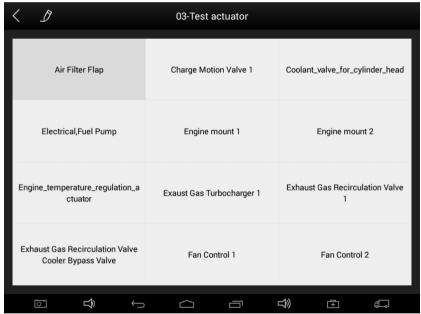
Tip: **Actuating Components Test** performs function tests for system components. When performing this function, the diagnostic tool will simulate the ECU signal to enable the user to judge whether the actuating components or circuits are working correctly.
