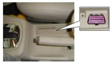
\*VW Passat B5: the OBD plug is behind the gearlever and beside the parking brake lever. Lift the cover to access it. Use SMART OBDII-16 connector.
