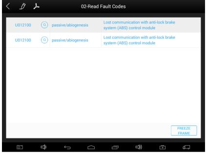
Tip: In the process of diagnosis, if the device shows "System is OK" or "No Trouble Code", it indicates that the ECU has not detected a fault in any of the circuits that it monitors. If there is a fault which is not being recorded it may be that the fault is with a part of the system not under the control of ECU, such as a mechanical system fault. It is also possible that the signal of a system sensor may be incorrect but still within the ECUs stored limits, this can be verified in Live Data.
