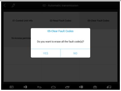
**4.5.2.** Click **YES** to confirm the operation, if the communication is normal, it will show "**Trouble Codes Successfully Cleared**" or "**Trouble Codes Cleared**". Generally, users will need to re-read trouble codes after clearing them to confirm that the trouble codes have been cleared.
