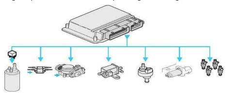
4.8.1. Return to **Dynamic Diagnostic Data**, enter **Test Actuator** and it will show the menu of the components that are available to actuate, shown below:
